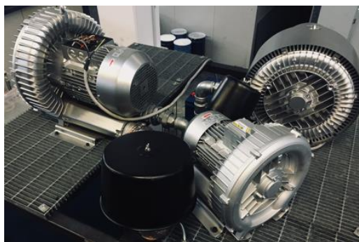
Figure 2. From the left: maon chamber with analogic pressure control, the installed blowers, the cabin for test confinement
