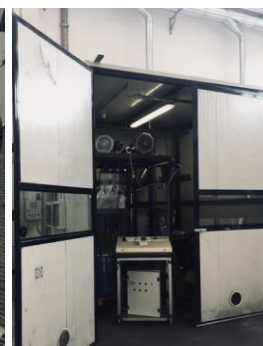
Figure 2. From the left: maon chamber with analogic pressure control, the installed blowers, the cabin for test confinement
