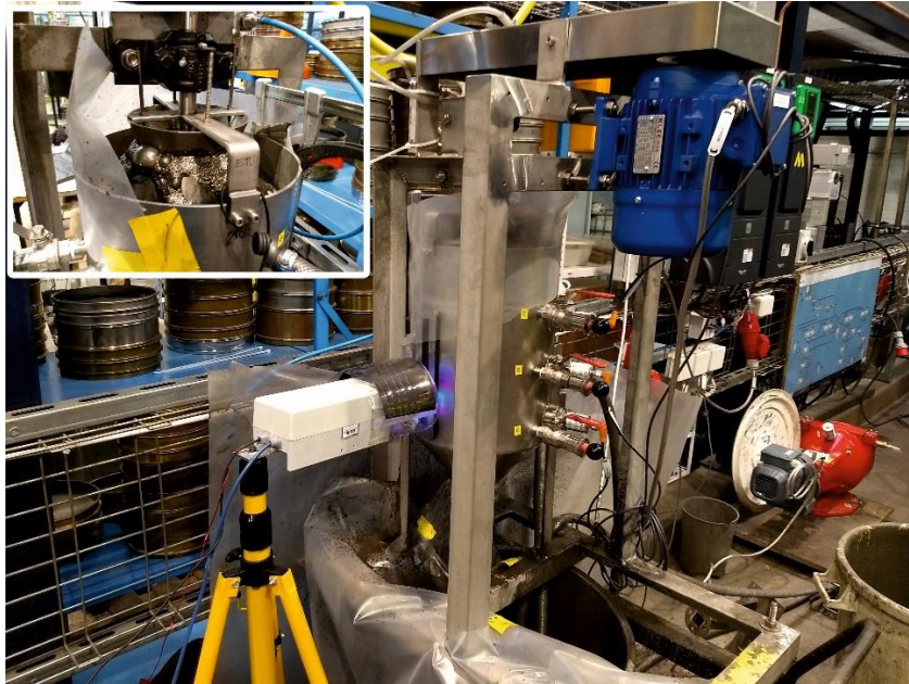
Figure 15. Coarse flotation device in minipilot-scale. On top, a copper concentrate is flowing from the top of the device. In the lower left corner, the particle tracking measurement device is also seen.
