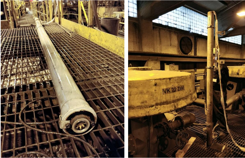
Figure 17. a) Measurement device: a machine vision camera with a ring of white LEDs around the lens inside a long waterproof housing; b) Measurement device inserted into the flotation cell through a hole in the grate.
