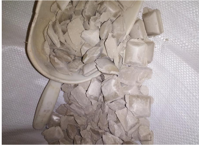
Figure 8. Pelletized material resulting from the rolling compaction stage of the Manfredini Fusion system.
